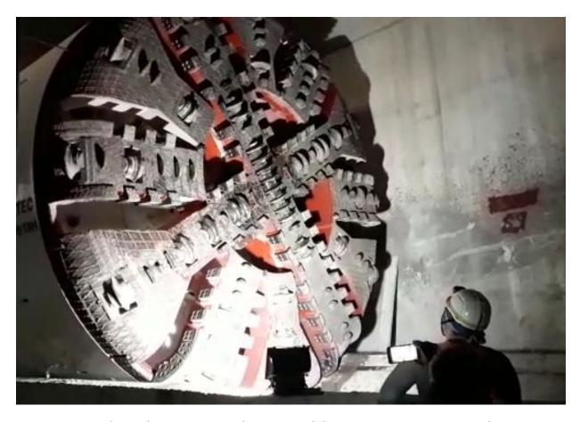
TERRATEC is pleased to announce the successful site acceptance testing of two new 6.56m diameter Earth Pressure Balance Tunnel Boring Machines (EPBMs) for the ongoing expansion of Istanbul's Metro system, in Turkey. These EPBMs, along with another two new sister machines that have been delivered to this project, will bring the number of TERRATEC machines working on the city's metro to a total of seven.
